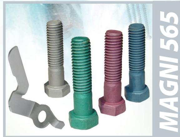
Magni 565 is a chrome free duplex fastener coating system that combines an inorganic zinc-rich basecoat with an aluminum-rich organic topcoat.
